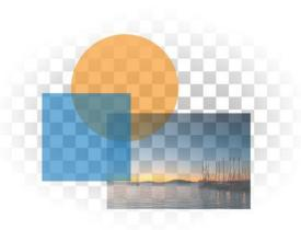
Alpha blending allows the rendering of high quality antialiased graphical elements and images by allowing edge antialiasing through semitransparent pixels.
