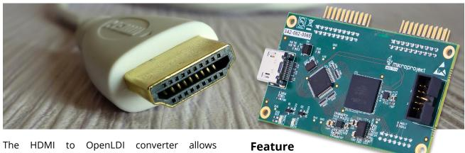
developers to easily interface the Intel Max 10 FPGA with HDMI streaming video, supporting the conversion of video resolutions up to 1080p60 to dual link OpenLDI.
